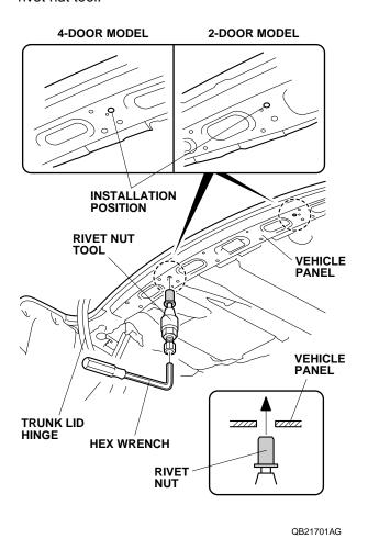
3. While holding the rivet nut tool with the hex wrench, turn the 19 mm wrench counterclockwise and install the rivet nut to the vehicle panel.
